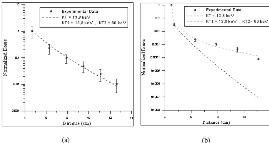
**FIGURE 4.** Dose-distance dependence for electrons traveling in air (a), for electrons traveling in air and aluminium (b); in this last case the TLDs were covered with a different number of aluminium foils of 50  $\mu\text{m}$  thickness.
