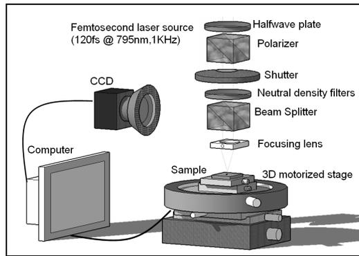
**FIGURE 1.** Experimental setup: a CPA laser with  $E = 900\mu J$  and 110 fs is focused by an optical bench onto a solid target of aluminium placed into a 3D motorized translation stage. The focusing system is a microscope objective 10x NA = 0.25. The focal spot has a radius of  $r = 3.8 \mu m$  resulting an intensity of  $I = 1.7 \times 10^{16} \text{ W/cm}^2$ .
