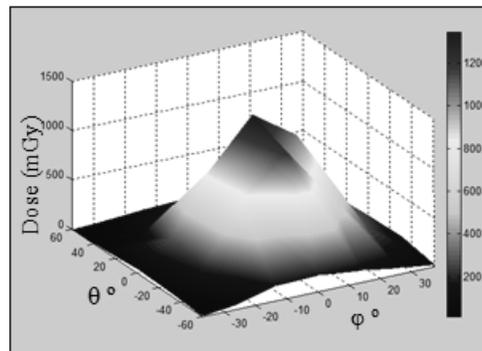
**FIGURE 3.** Angular distribution of the emitted radiation in the case of  $p$ -polarized laser pulses.
